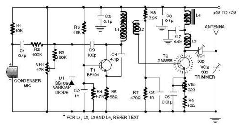
The transmitter circuit described here has an extra RF power amplifier stage, after the oscillator stage, to raise the power output to 200-250 milliwatts. With a good matching 50-ohm ground plane antenna or multi-element Yagi antenna, this transmitter can provide reasonably good signal strength up to a distance of about 2 kilometres.
